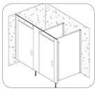
**FLOOR-MOUNTED OVERHEAD-BRACED** Strongest and most economical installation.
